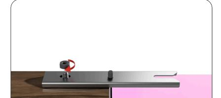
Screw adjustment coupler into Bridge Plate and hang baffle by threading loop cable into the adjustment coupler.
