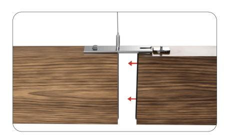
Place a small drop of Loctite on the second baffle's stud and screw a 1/4"x20 nut into place.
