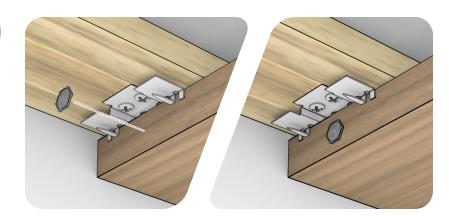
Only one bumpon spacer is needed for subsequent planks within the row. They should be inserted within 2" of the trailing end of the plank.
