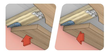
Lift the opposite edge of the plank against the base of the Plank Clip, then slide the plank (along with the Slotted Perimeter Clips) into the Plank Clip's prongs. 17
