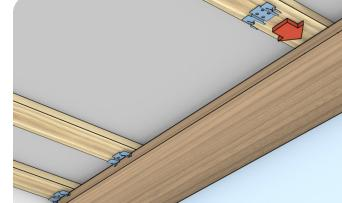
In many instances, measuring the installation locations and attaching the Plank Clips on the plank's outside edge before installing is an easier and faster process.
