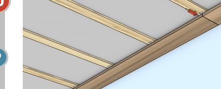
In many instances, inserting the bumpon spacer on the plank's outside edge before installing the plank is an easier and faster process.
