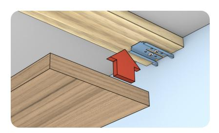
Slide plank into the prongs of the Slotted Perimeter Clip.
