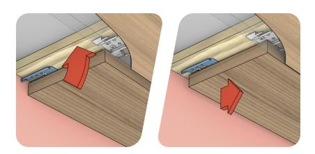
Continue installing the final row of planks, following the previous steps 16 – 17, until all the planks are installed.
