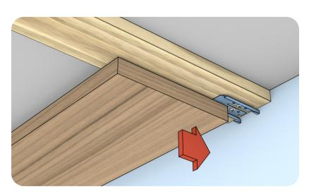
Ensure plank is fully seated against the back of the prongs.
