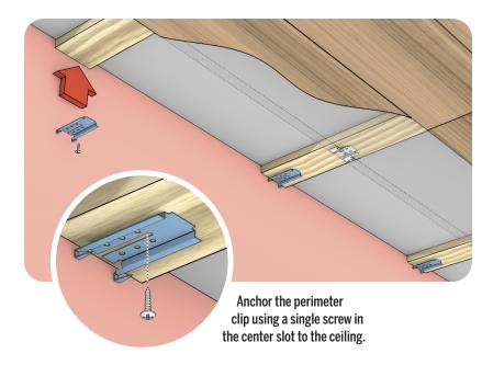
Keep the screw loose enough to allow the clip to slide within the slot. W .
