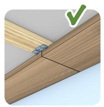
With the Plank Clip's prongs fully inserted, use two screws to fasten the clip to the furring strip.
